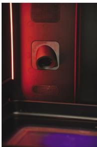
Origin One features several integrated cameras for computer vision and capturing temperature data in the IR range; additional sensors measure other environmental conditions during the print process.
